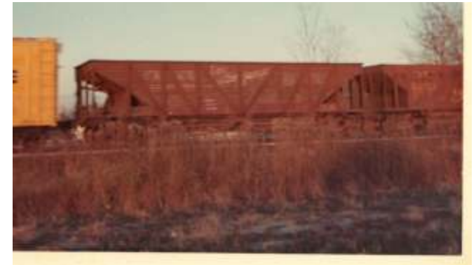
A Prototype. A style of composite railcar is this CB&Q Ballast Hopper in Chicago Ridge about 1974. Photo ©Rob Manley
