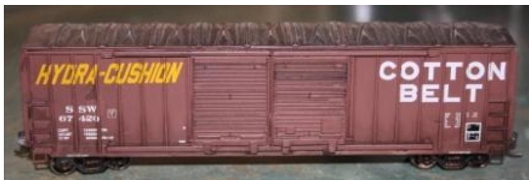
Things to look for on your first coaches or freight cars are; free spinning wheel sets, metal wheel treads, free swinging bogies, freely operating couplers and a uniform weight per unit length.
