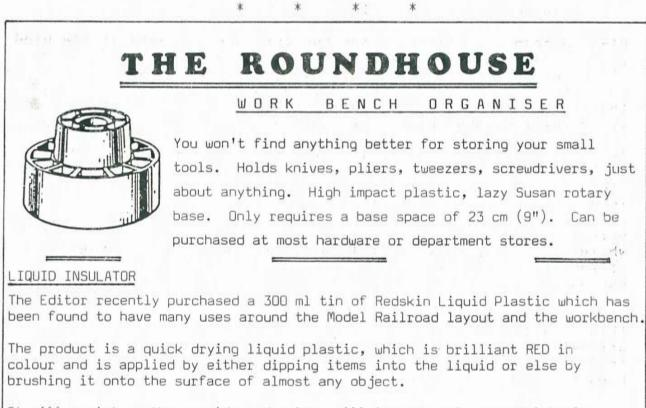
It will resist weather, acids and salts, will improve grip on metal tools, insulate bare wires and electrical connections and the colour will easily identify an item from a distance. Dangerous can or bottle contents can be sealed in safely and generally it can be peeled off most surfaces.
