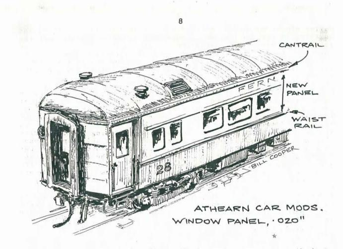
The main body was made first. Window shapes were scribed; t corners drilled and then cut out with a jewellers'saw (followi DAW's dictum '..measure twice and cut once..') Several saw blad later (thank Heaven hardware stores stay open on Saturday now) t blanks were ready for filing. Filing just three window shapes to precise size indicated the folly of attempting to cut masses of them in car sides, though this has been advocated in some English articles. They must have long winters...
