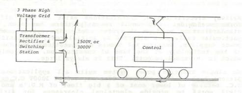
Double End Feeding enables the train load to be fed by effectively two paths and so the individual wiring currents are reduced. Substations may be at up to 20 kilometres spacings.
