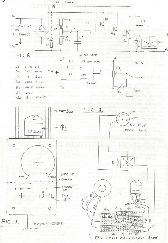
switch as shown in fig **2** and the BLUE and WHITE wire to the circuit board at points AC. There is no polarity with blue and white so you can connect them which ever way you like. If the red / black are connected wrongly then the train will travel in the direction OPPOSITE to the switch. [Murphy's Law states "if there is a 50/50 chance of connecting the wires right, you will get it wrong ---90% of the time!!!]
