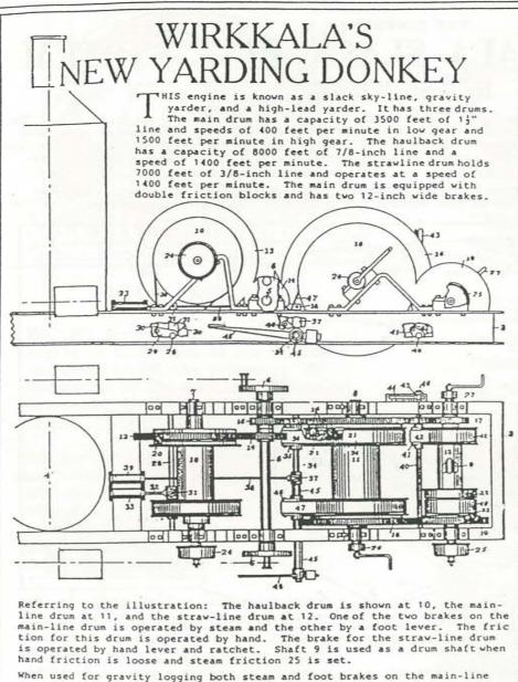
When used for gravity logging both steam and foot brakes on the main-lid drum are used, while for other purposes the foot brake alone is used.
