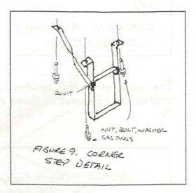
Make the corner steps of .010 by scale 3" wide flat brass strip and solder or glue thern together and attach to the car. I drilled small holes in the mounting areas of the steps, glued the steps to the car, then
