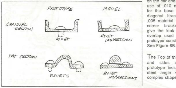
FIGURET CHANNEL AND HAT SECTION CONSTRUCTION diagonal brace flanges on the car ends. The use of .010 material for the base of the diagonal brace and .005 material for the corner bracket will give the look of the overlap used in the prototype construction.
