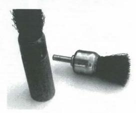
brush. It is the type you put into a power drill. The brass wires are very close and
