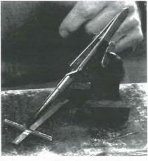
end pressure of the tweezers [locked into the 3rd hand] on top of the pieces to be soldered. Because in this technique you do not need to touch the pieces to be soldered you will only need enough pressure to stabilise the work piece, which requires very little pressure]
