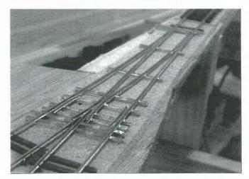
The track is pinned down every 100mm or so with 15mm x 1mm panel pins with their heads cut off-Oooooh! Good metal straight edges are use for the straight bits and the usual easements are used on curves.
