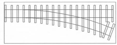
a template is to photocopy a commercial turnout. If you model, say On3, you can photocopy an HO standard-gauge turnout and enlarge it by 115% to get a fairly good On3 template. To calculate this percentage, just divide the gauge you want (On3 is 19mm) by the sample you have (in this case an HO gauge of 16.5 mm). Multiply the result by 100 to get a % figure. You will have to ignore the ties, but it will give you an accurate gauge and position of the rails, frog, guardrails and the turnout blades.
