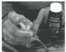
Apply flux with a needle
