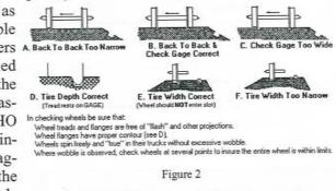
"B" figure 2. I am assuming you have already changed to metal wheels so it is usually a simple matter of removing the axle from the truck, holding a wheel in each hand, twisting at the same time as pulling or pushing repeatedly until they fit the gauge slots. In
