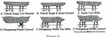
Frogs are checked with the "FLANGEWAYS" side of the gauge. Application of light side pressure toward the frog against the Guard Rail (see D.Flangeway Depth Correct arrow). Figure 4 shows the interpretation of the Figure 4 results. Gauge prongs must clear all obstructions below the rail head as in D. Use "NO-GO" side prong of Gauge to check Flangeway width at the Frog in E and F.
