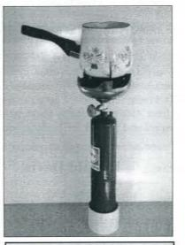
Photograph 2: The gas bottle, heating ring and pot ready for use
