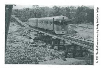
2028 Mt. Surprise powered by two Rolls Royce diesel engines.
