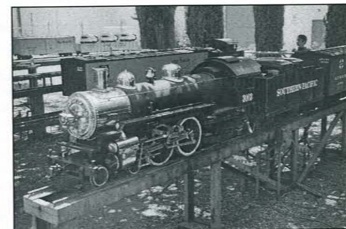
Southern Pacific Baldwin 4-4-2. Seen at Riverside Live Steamers, Riverside, California.
