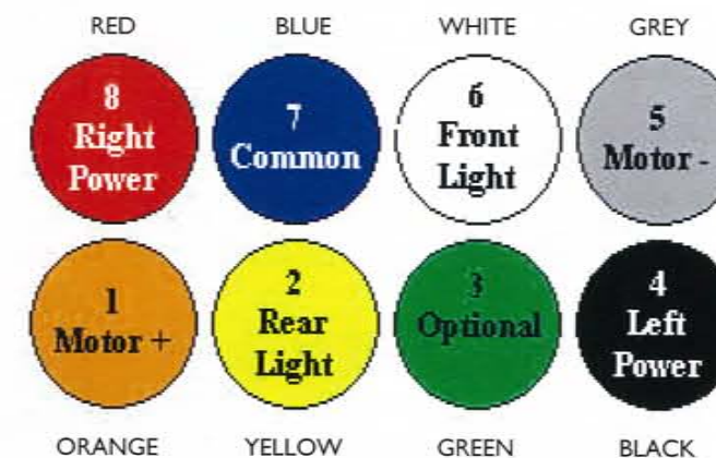
Above: NMRA standard 8 pin decoder plug wiring arrangement (view looking into the socket from the plug) NB the colours of the wires are the same as the diagram at the top. The plug is just an easy way to connect your decoder to the locomotive without soldering required. (Provided the locomotive circuit board supports this plug)
