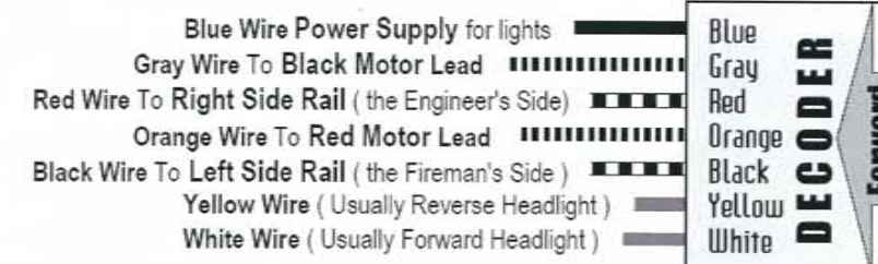
Above: General wiring diagram of a standard NMRA compliant decoder
