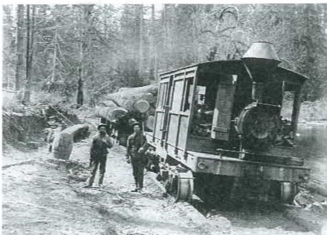
Early Climax Locomotive fitted with concave wheels. This type of locomotive was referred to as a "Pole Road Climax"
