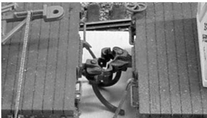
Image One shows the coupler being separated. This can be done with 'twisle stick' as shown or with magnet.
