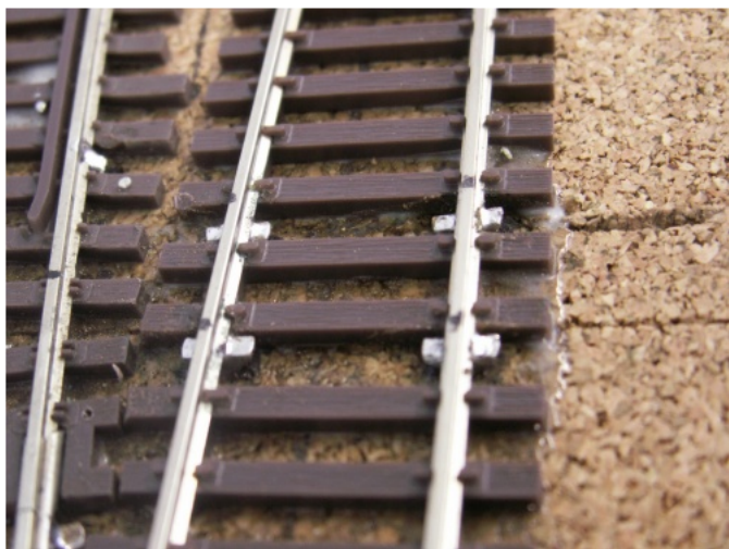
Photo 3 - Track joins at the ends of modules. This is done using small brass screws soldered to the rails and track ties are glued to the Cork roadbed. These will be then cut with a razor saw.
