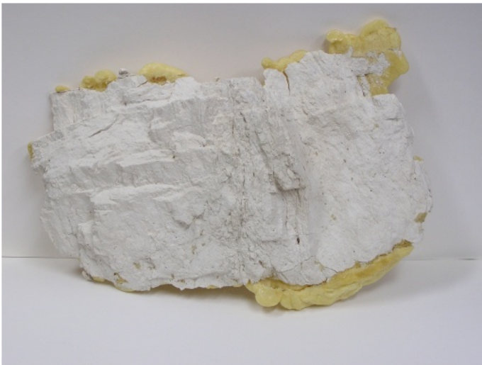
Photo No. 6 Plaster casting with Polyurethane backing
