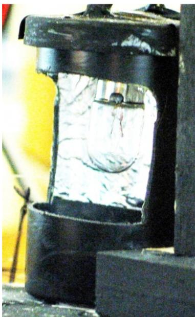
Figure 1 – The modified 35mm film canister with the “window” cut out.
