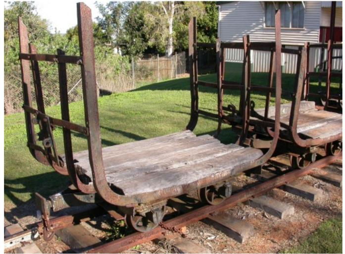
CSR metal 'basket' type wholestick trucks at the Childers Museum, 2006. A chain or rope was thrown over the top and winched tight to hold the load. These trucks were not measured but the dimensions are likely fairly close to the Fijian truck measured by John Teichmoeller in 1963. The timber has been added for health and safety reasons and were not necessarily used when the trucks were in service. Lynn Zelmer photo.
