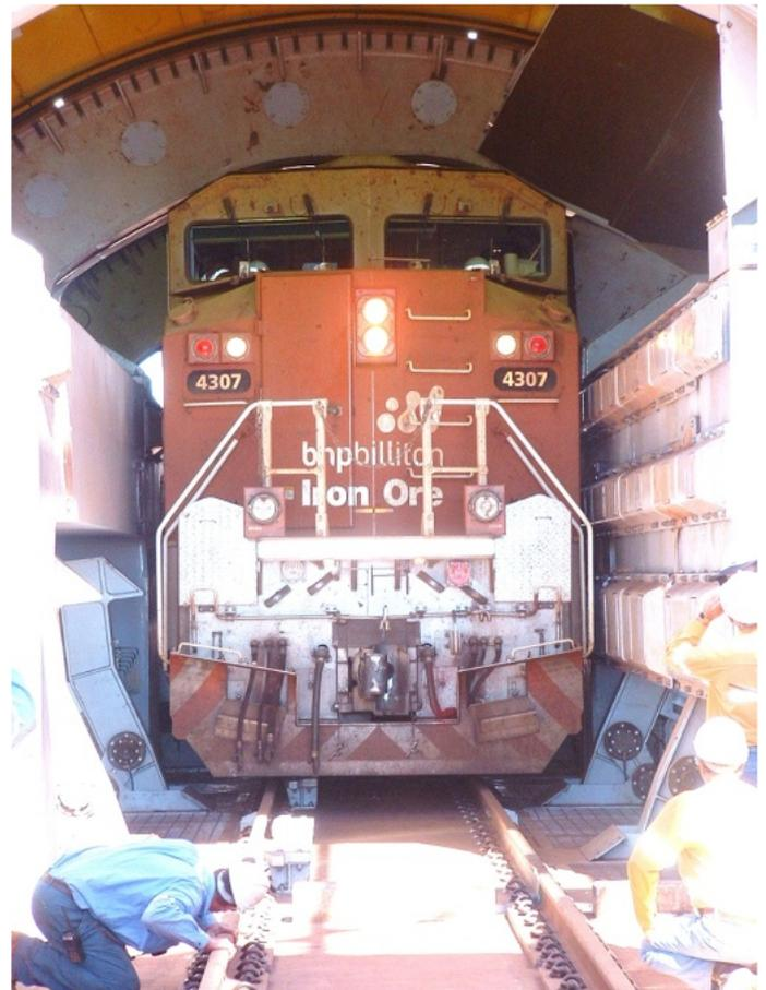
This article shows a test train used to check the cow catcher to the wheel locks. This required a fully loaded locomotive with rolling elements that were nearing their useful life. i.e. worn wheels. Once clearance is confirmed the wheel chocks are grouted into place.
