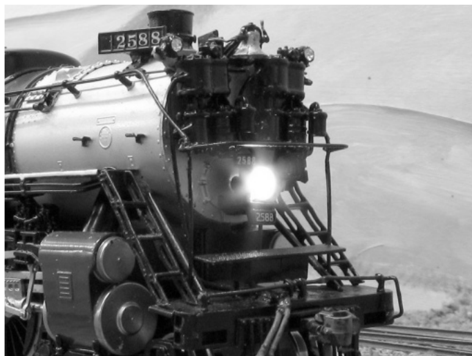
SMD LED used in the Headlight of brass loco.
