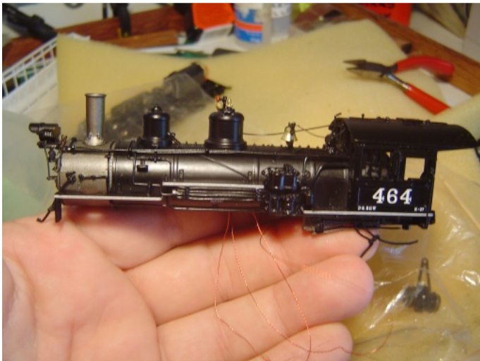
Routing wires through boiler
