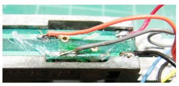
You can finish here if you wish, and just cut the 3 other wires short and refit the body. I chose to add the head lights using the same method as for the 44 class. This time I used  $2 \times 0.75$  mm fibre optics from the one LED.
