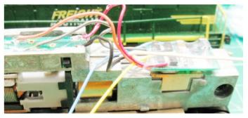
In all cases I use 820 ohm resistors for this type of application. Remember the longer lead on the LED goes to the Blue wire from the decoder.
