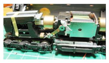
The motor is turned on its side because of height restrictions but still fits in the wide body locos such as the BL class, GM class and the 442 class.
