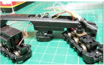
Unclip the body and remove. You will see a printed circuit board on top of the chassis – two wires from the pickups on the front truck and then two wires going to the motor. The most important thing is the slot in the metal weight under the board. Place the decoder in the slot (with the wires facing forward) and place a small piece of sticky tape over the top to hold in place while you are working.
