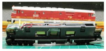
The decoder fits in the little recess at one end and the wires fit between the two halves of the chassis. You have to take the chassis apart to solder the wires to the motor terminals. Make sure the brush posts do not touch the frame - a little grinding may be called for here. There was no way of fitting lights to this loco as there is a lot of resin on the wall behind the lights - it is just not practical.
