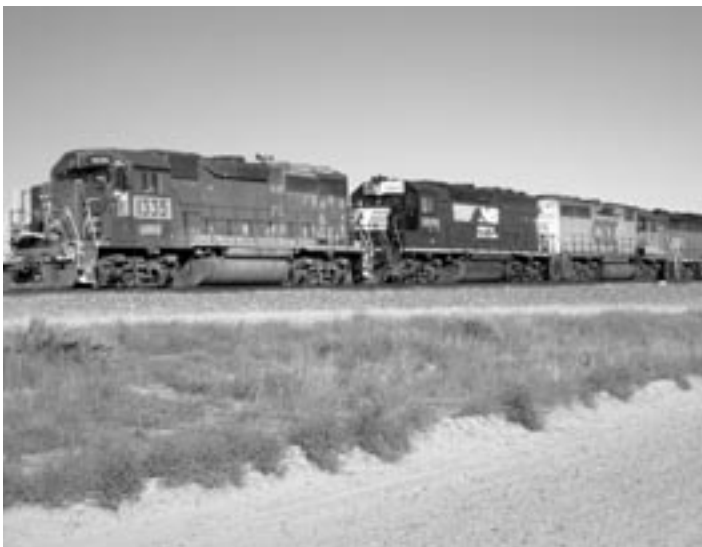
These well-worn lcomotives are provided by the class 1 railroads. They are used to pull heavy trains on the four kilometer High Tonnage Loop (HTL). Test train operations are designed to accumulate 1 million gross ton traffic density per day at a maximum operating speed of 40mph (64 km/h). The HTL is used for research on track component reliability, wear and fatigue.
