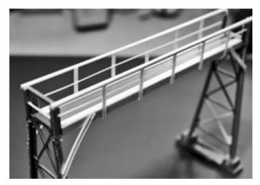
We need at least 5 fence post locations equally spaced along each side of the walkway. Measure and mark along the edge of the walkway five equally spaced fence post locations. Once you have completed this step, use a small toolmaker's square to mark the same post locations on the other side of the walkway.
