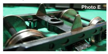
The next photo shows the simple modification that will allow the truck to rock from side to side – not much but enough to keep the coach on the track.
