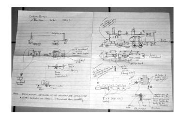
During the disassembly process, any faults found can be addressed. I generally draw up a diagram during disassembly. Please do this over a tray, so that any screws and small parts don't escape. Put these into a plastic bag. Note - complete disassembly is not required, just take the unit back to subassemblies.
