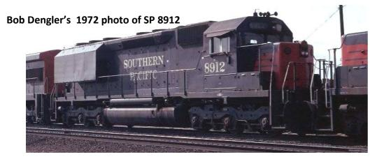
One of my long term modelling aims was to modify an SD45 to resemble the units Southern Pacific fitted with radiator inlet shrouds. The shrouds prevented hot air being sucked into the radiators while operating up grade at full power in long tunnels. The hot air sucked into the radiators caused the engine to over heat and shut down the locomotive
