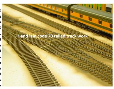
Switchmaster but a few Tortoise and Tam Valley servos. The wiring is straight forward with the droppers soldered to the bottom of the rail – looks tidy that way. Before sections were sceniced, the track was fully tested – with full trains and plenty of operation. A few minor changes were carried out but generally things were OK. All mainline turnouts are run by accessory decoders. I am now at the stage where I am motorizing the turnouts in the yards and switching areas all with servos.
