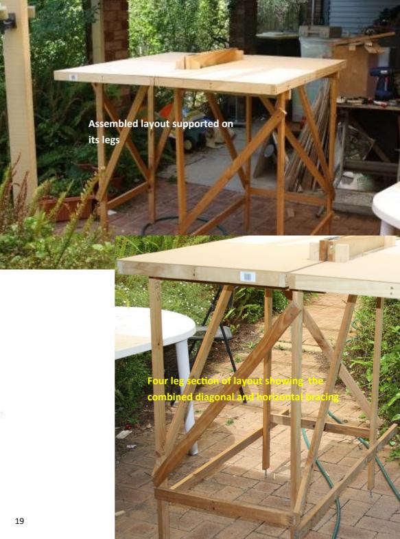
The two legged frame section's pair of legs are secured to the frame cross members. This places the legs less than 600 mm apart. To support the frame longitudinal side member at
