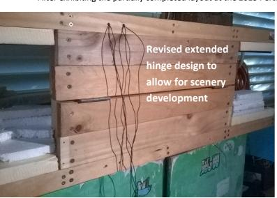
came apparent the hinge mountings were too low to allow reasonable scenery on both halves of the folding layout. I raised the hinge line by 68 mm. the hinge mounting boards are now secured to the layout framing by lengths of 68 mm by 19 mm pine
