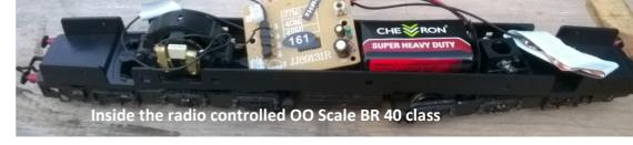
I tried two AA dry cell batteries but they wouldn't budge the Lima motor. In desperation I tried a nine volt battery. This worked well. (No smoke!) With a little wriggling I installed the receiver circuit board from the pickup, the nine volt battery and the attendant wiring into the 40 class and reinstalled the body shell. On the layout the model sailed along at a sedate speed. This was a considerable improvement on my previous attempts to operate this model on DC track power. I was in business.
