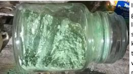
I blended a jar of dry plaster of Paris, some green tempura paint powder and a little yellow oxide to what seemed to be a reasonable shade of green grass and gave it a go. I sprinkled the coloured plaster mix over damp plaster coated scenery from a tea strainer and waited for it to set. Inspecting the results the next morning showed the coloured plaster
