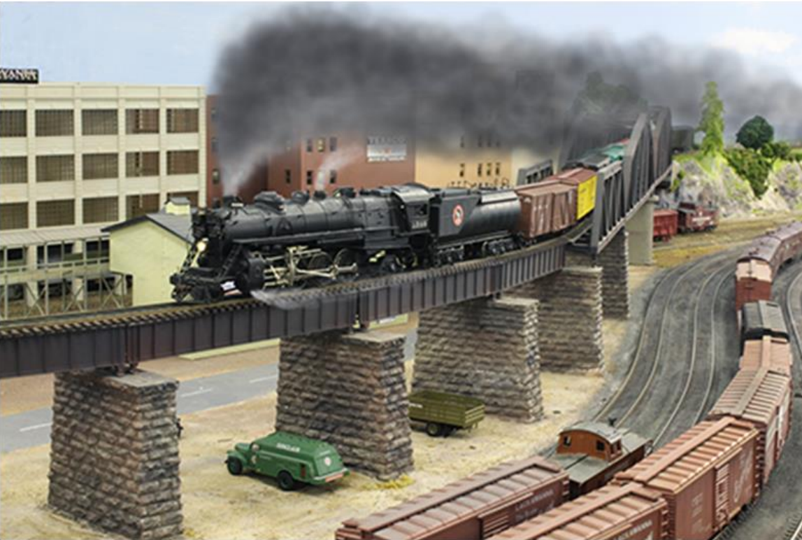
Great Northern 3399 fitted with a can motor, the speaker installed in the boiler, a current keeper and a Tsunami 2 decoder crosses the 3 rd street viaduct on a test run on the West Ely branch. Photo by Charles Page.
