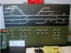
termining what trains need to be run. The Yardmaster is the controller of the Coburg Yard, and this does not appear on the Dispatchers control panel, as he is not concerned with what goes on inside yard limits. The CTC system was built using 4 SMINI nodes and 9 block detectors from Bruce Chubb MMR. Kelly Loyd programmed the system on the computer. There is
