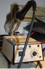
9 Soldering Iron – 40 watt minimum – with fine tip. Temp control would also be good. You would need to set it at 280 C. \$60.00
