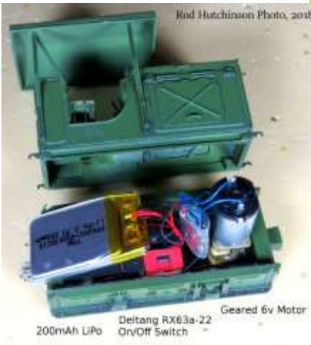
Under the bonnet of Rod Hutchinson's Malcolm More rail tractor
