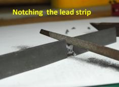
Step 4: Cutting out the notches in the lead sheet to fit around the exhaust stacks. I did this with a small triangle file, after marking the position where the notches were required
