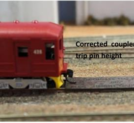
Next was a coupler height check. Oh dear one end was really low!!! This was readily corrected by bending the coupler glad hand upwards.
