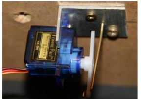
The motors are supplied with a selection of armatures, a small screw to fix the armature to the motor shaft, and two slightly larger screws to use in mounting the motor. I used one of these screws to hold the motor to the bracket.
