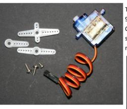
I also picked up a Servo Shield which plugs directly on top of the Mega. This shield board makes it easy to connect the servo motors and can connect a dozen at once if The Servo motor I used was the Tower Pro Micro Servo 9G, model SG90. These are small, light weight and CHEAP, and come complete with connecting cable and a selection of control arms. I picked up a dozen for not much from Ebay.
