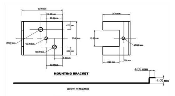
The two larger holes in the Aluminium bracket are used to mount the switch machine. I mounted one to a sample board using 10mm long wood screws.
