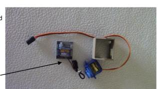
brackets for point servos for his layout. These are handy where below the base board mounting was found to be difficult. Tower Pro SD90 & S361 Hobby King Micro servos here shown in to David's 3D printed mounting bases
