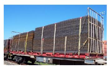
1 Has end gates & secured by 5t Web Straps
