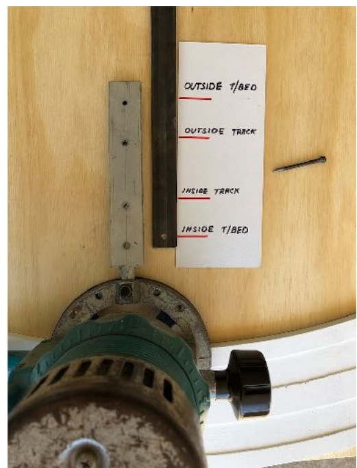
5 Showing Router with Radial Arm Attachment & Positioning Points
