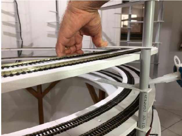
15 Secure steel support bracket to trackbed with a bead of Silicon
