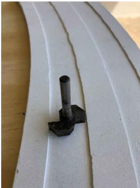
6 31mm Router Blade used for cutting trackbed recess
