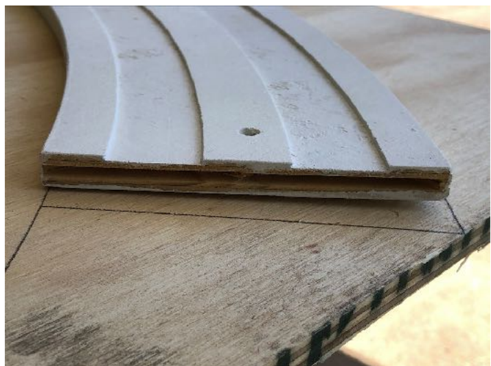
7 Biscuit cuts in end of the Trackbed Sections
