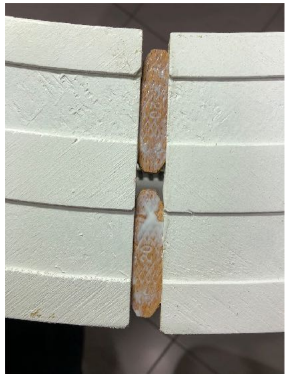
11 Glue Trackbed sections together with two #20 Wood Joining Biscuits
