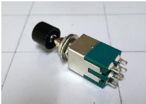
1 A DPDT (constant on) Push Button Switch used to switch the Turnouts
