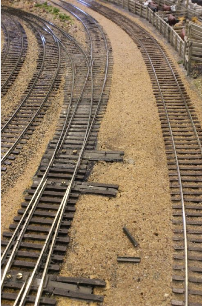
16 Customised Code 70 L/H Curved turnout hand laid between a modified Shinohara R/H curved turnout and a modified three way turnout.
