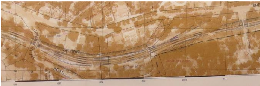
6 Portion of topographical map showing station area with tracks and two overbridges (note that this map is earlier than the 1980s and shows the earlier track arrangement, with three through roads and sidings for suburban locomotive servicing)
