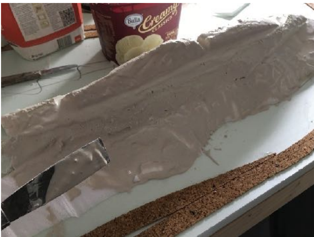
10 Plaster being applied with a spatula
