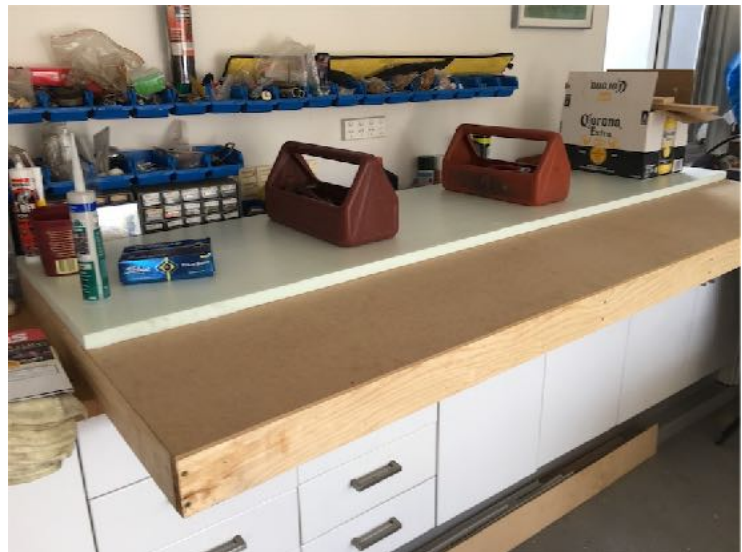
2 Base with EPS Form Sheet attached
