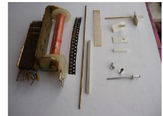
Cut the 1mm thick styrene sheet to a scale  $10ft \times 5ft (20mm \times 10mm)$  size. This is the base on which to mount the signal and will be covered with dirt etc.
