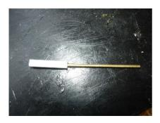
Glue the brass tube into the styrene tube flush with the bottom.
