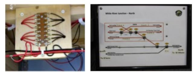
Learn how to make very easy to understand control panels. Easy to read locations and track diagrams. This one is nicely mounted in a photo frame. There is a hinge on the bottom so that the panel can be folded forward for easy access to the wiring.
