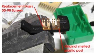
the diameter of the holes in the wipers and they neatly fit a 00-90 screw (good news for N-scalers – exactly what you use for your MicroTrains couplers). So, already being equipped with the drill and tap for couplers, off I went. The result is shown in Photo 1 and so far performs faultlessly. It looks as if I shall have a rainy day devoted to fixing the other dozen. It would also be possible to use very small self-tapping screws if you don't already have the tap.
