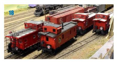
With all the lights at the front of the trains, each caboose has the red marker lights 18. Some of these also have interior lights controlled by old loco decoders so the lights can be turned on and off. There were very few suitable cabooses around so a number were repainted and the "old" Athearn cabooses had
