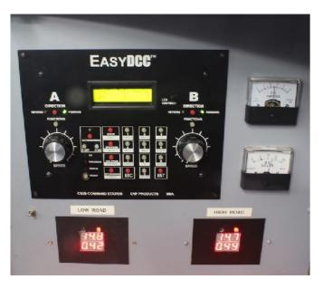
voltage of 14.6 volts. This is verified by two Rampmeters that give constant readings of the power buss. A computer is connected to the command station and runs a program JMRI which has many sub systems for model railroaders. I use one - Decoder Pro, this is for testing and programming the decoders in each of the locos. The computer is also connected to a programme track through a Sprog 3 unit.
