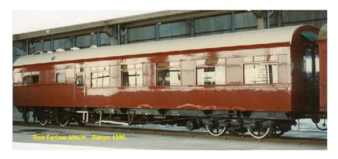
In 1970, cars 1255 and 1256 were converted to Griddle Car. The kitchen area was extended to make a servery, gas bottles were added reducing seating from 30 to 22. These wooden cars were used on special trains that ran and
