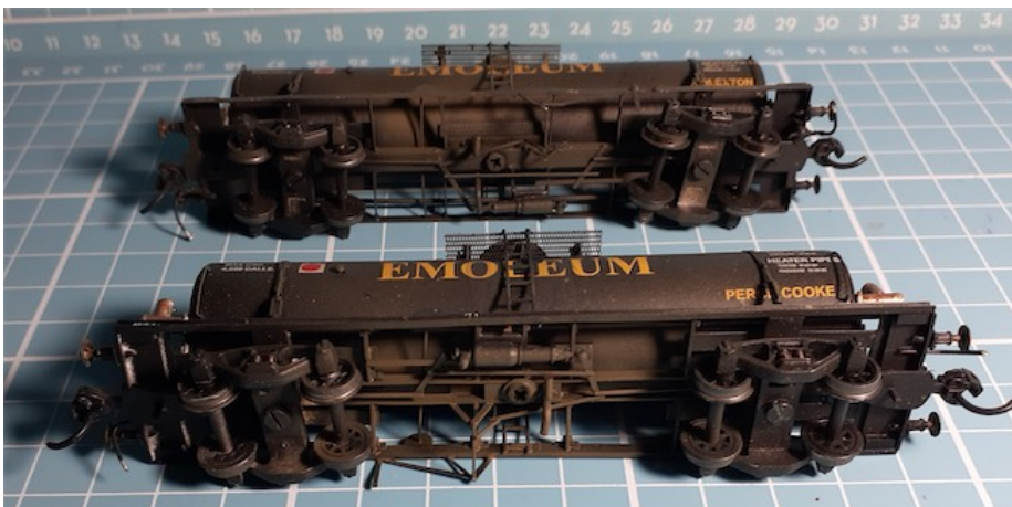
Brake rigging and under frame detail was added to complete the car.
