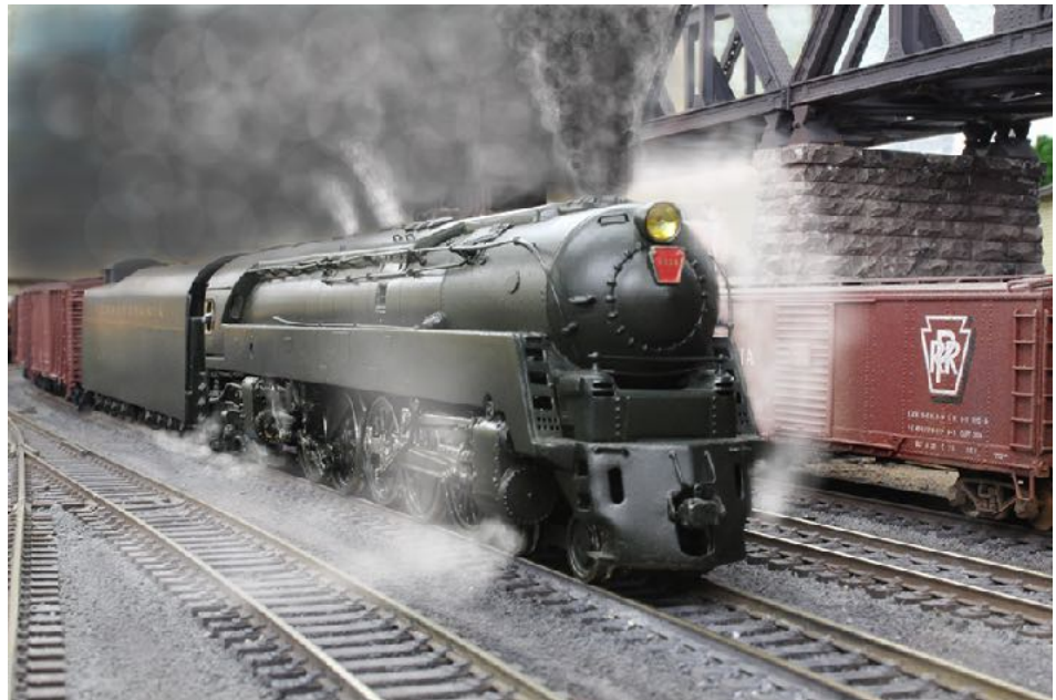
The Q1 is a 4-6-4-4 one off duplex designed for fast freight service, (notice that the second set of cylinders are rear facing). It is departing Mount Loewy, Eastbound
