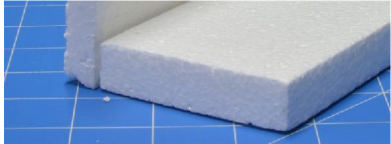
Photo 24 - Avoid this type of joint if possible
