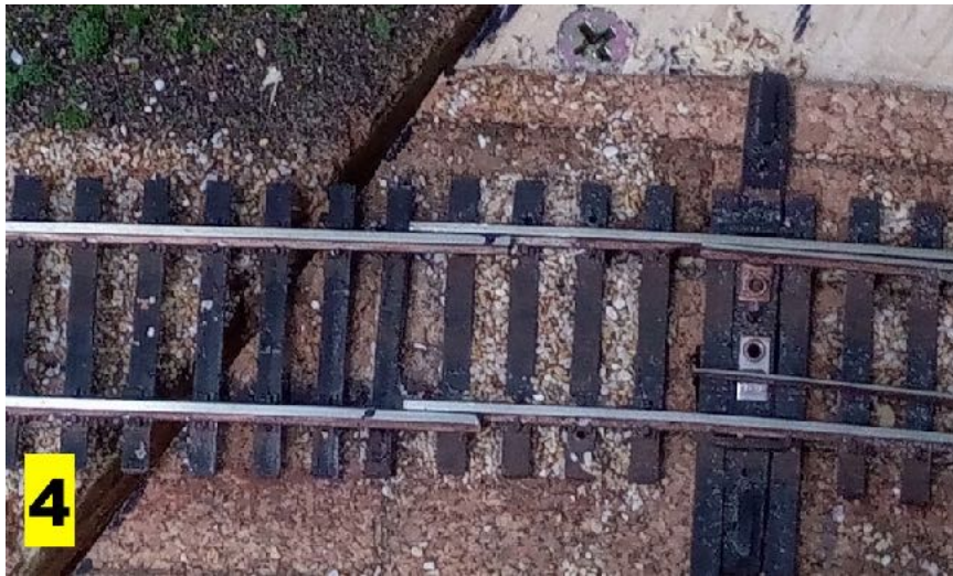
[4] Still need to do the final rail cut and then add joiners.
