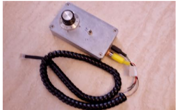
Jack Child's DC/DCC Throttle which can be plugged into NCE DCC panels
