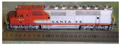
American rolling stock are around 35 mm wide by 67 mm tall. The photo of Santa Fe FP45 5947 gives an idea of the size of a HO scale model of a reasonably sized locomotive.
