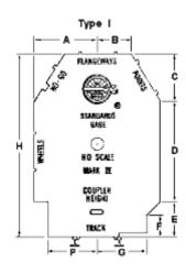
The horizontal and vertical clearances from the track centre line depend on the era and location you model and the curve radius you choose. NMRA S7 provides a range of clearances on straight track depending on era modelled. Details of NMRA S7 are shown on the NMRA web site (http://www.nmra.org/) The NMRA Standards gauge is a handy way of checking clearances on your layout
