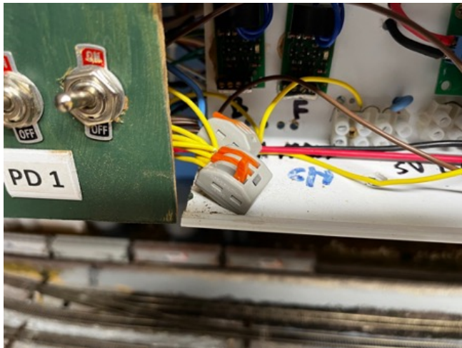
Fig 9: Connection to 5 volt bus and fascia switch via WAGO connector.
