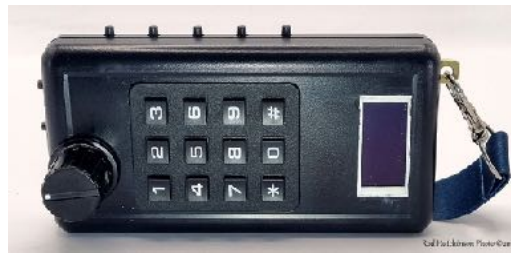
Philip Hillebrand: DCC-EX WiFi Throttle. (Under Development)
