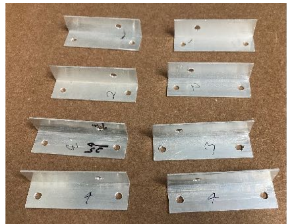
Left: Drilled leg and strut connection brackets.
