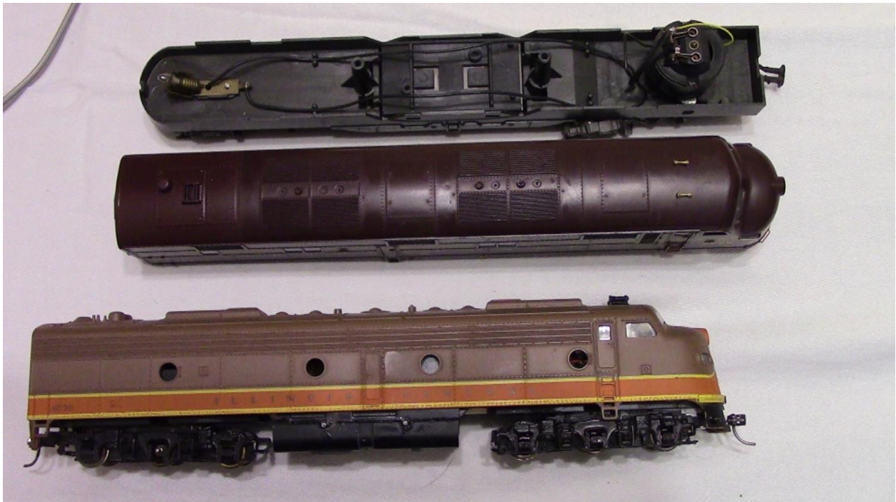
Top: Rivarossi chassis & motor. Centre: Top of shell. Below: E7 mechanism on the shell
