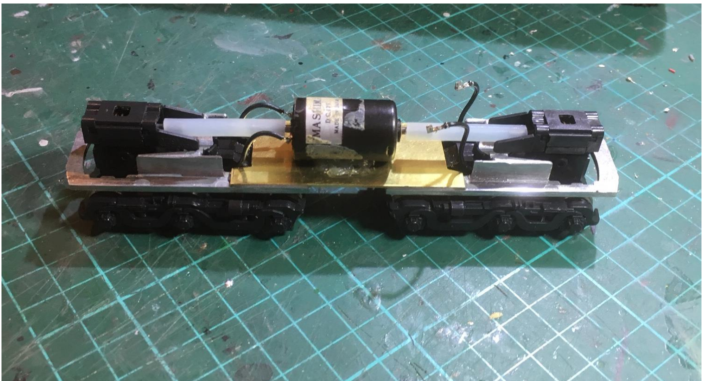
'New chassis' shows the shortened RSD-12 chassis with brass connecting plate.
